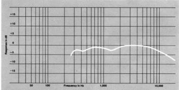
Frequency response contour of Model 2441 coupled to a 2350 horn. Measured response of a typical production unit, including all peaks and dips, does not deviate more than 2 dB from the above curve
